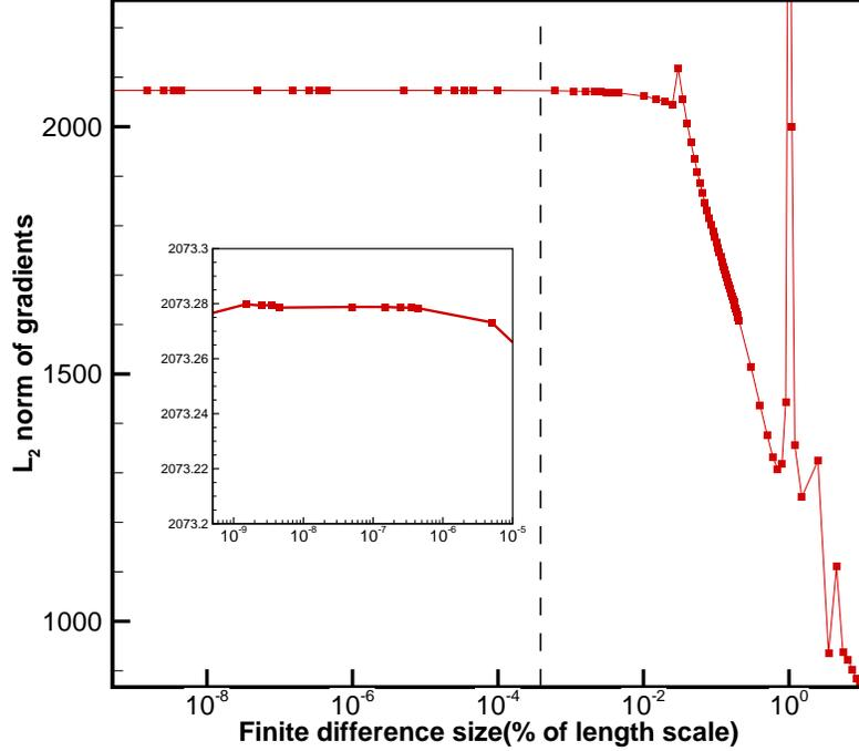
Figure 1: Sensitivity map of the gradient of the Jacobian matrix with respect to perturbation parameters for an inviscid Burgers' problem
