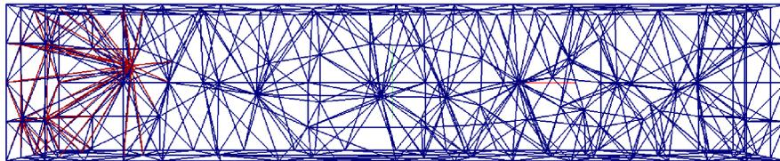
Figure 4: Mesh modification to stabilize the problem for a 3D  $2^{nd}$  order MUSCL advection
