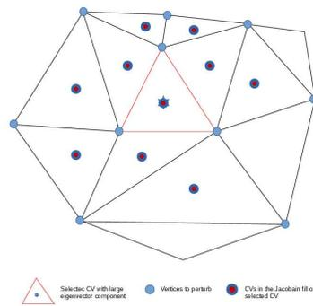
(b) Vertices on the control volumes of the Jacobian fill of the control volume with the largest eigenvector component
