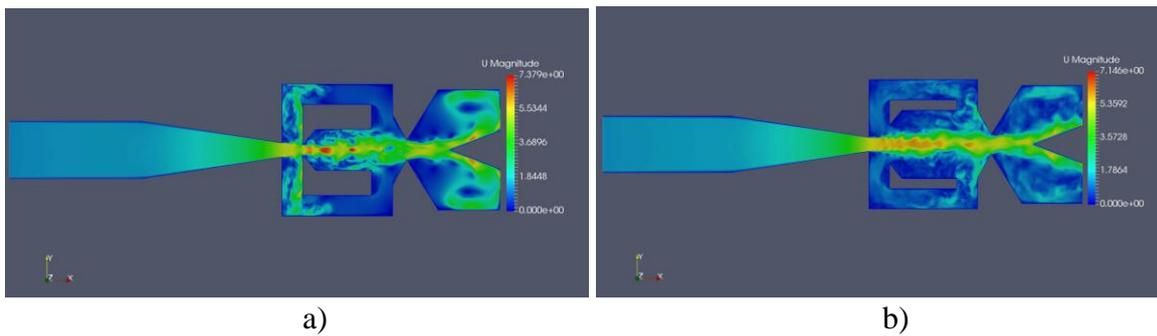
Fig 9 Fluidic amplifier internal flow visualization for a) minimum inlet width, b) maximum inlet width.
