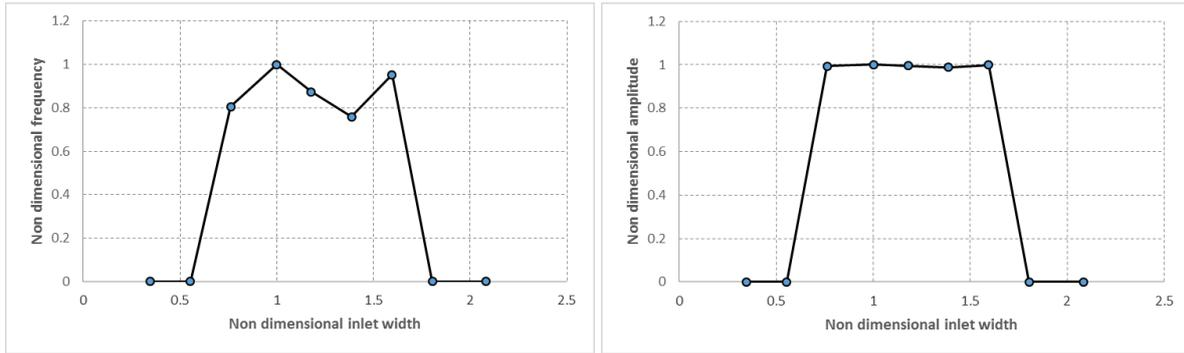
Fig 8 Non dimensional frequency and amplitude variation as a function of the mixing chamber inlet width.
