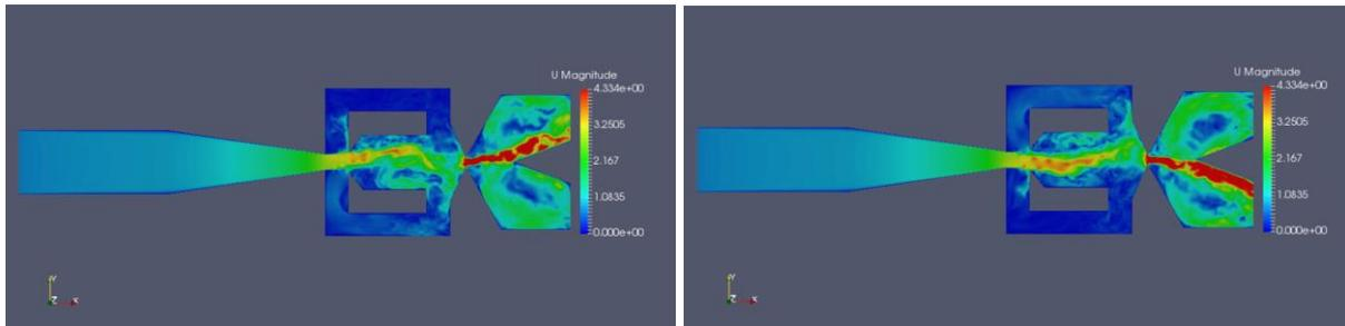
Fig 7 Fluidic amplifier internal flow visualization for the smallest outlet width studied.
