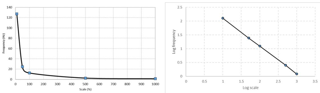
Fig 10 Variation of frequency when the fluidic actuator is scaled while maintaining constant the inlet Reynolds number.
