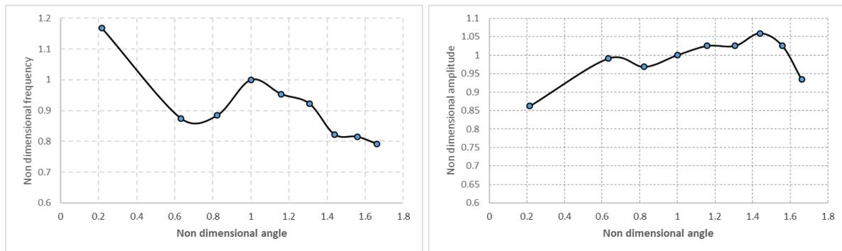
Fig 4 Non dimensional frequency and amplitude variation as a function of the mixing chamber outlet angle.
