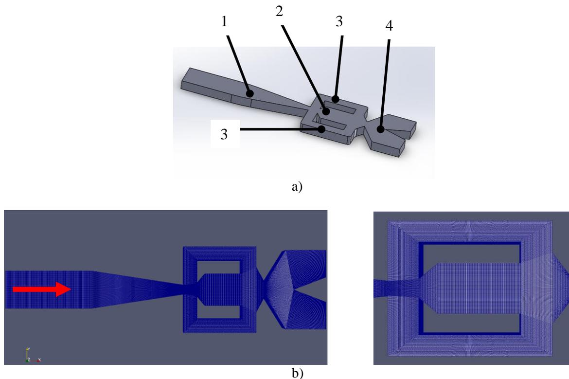
Fig 1 a) Main view of the fluidic actuator. b) Grid used in the present study and zoomed view of it.
