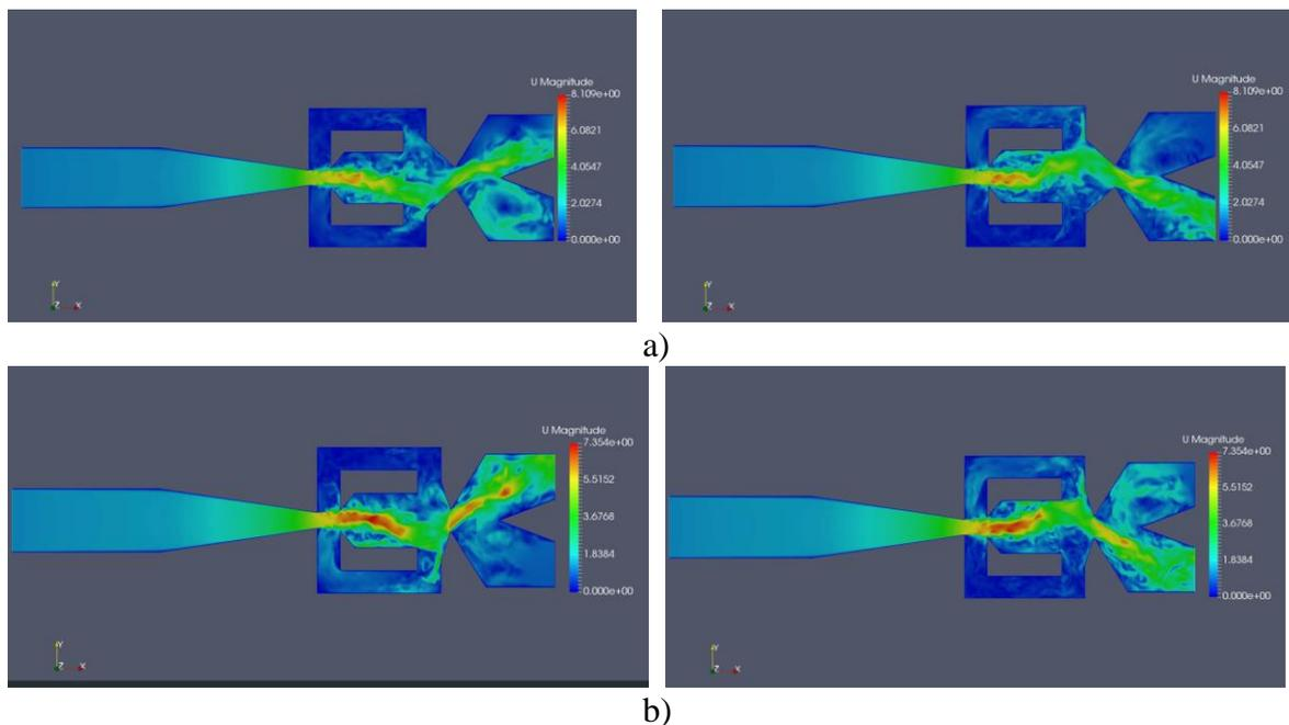
Fig 5 Fluidic amplifier internal flow visualization for a) maximum angle studied, b) minimum angle.
