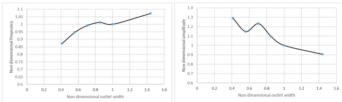
Fig 6 Non dimensional frequency and amplitude variation as a function of the mixing chamber outlet width.
