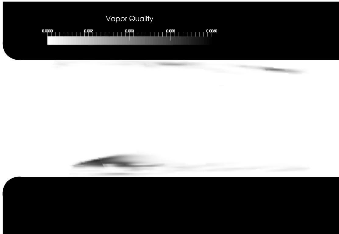
Figure 16: Cavitation inside the throttle. Pitch black area shows the throttle wall. The gray-scale represents the vapor mass fraction for this slightly cavitating flow
