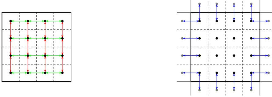
Figure 2: Inner-cell and over-interface reconstruction
