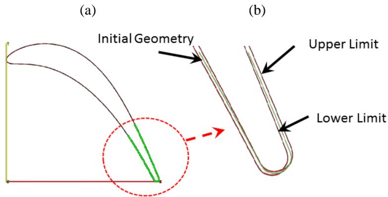
Figure 7. A) Source Points for Shape Deformation B) Upper and Lower Deformation Limits
