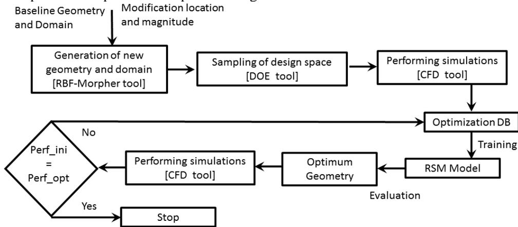
Figure 3. Algorithm of the RBF4AERO optimization process
