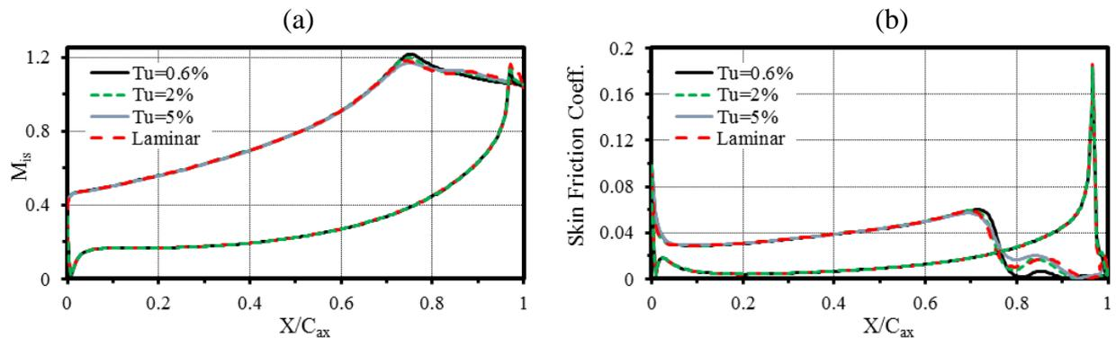
Figure 6. Effect of turbulence intensity a) Isentropic Mach Number b) Skin Friction Distribution
