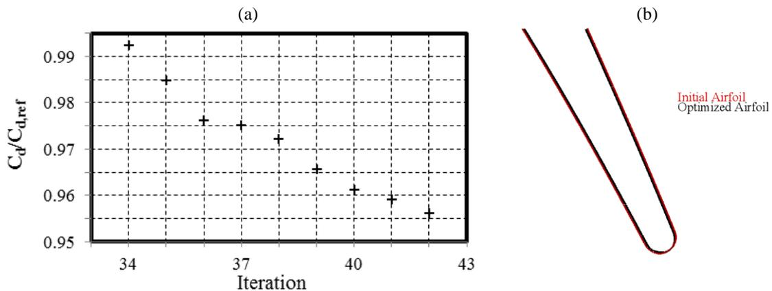
Figure 8. Comparison of initial and optimized airfoils a) Drag Coefficient Evolution b) Geometries
