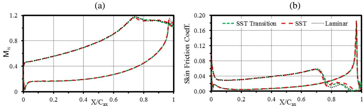
Figure 5. Effect of flow parameter on a) Isentropic Mach Number b) Skin Friction Distribution
