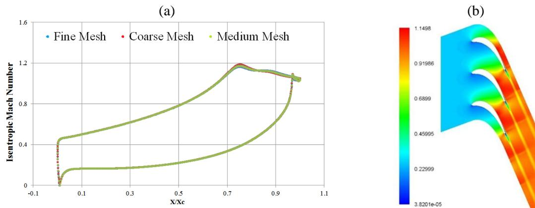
Figure 4. Isentropic Mach Number a) around the airfoil b) blade to blade contour
