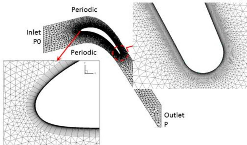
Figure 1. Mesh topology of the numerical domain
