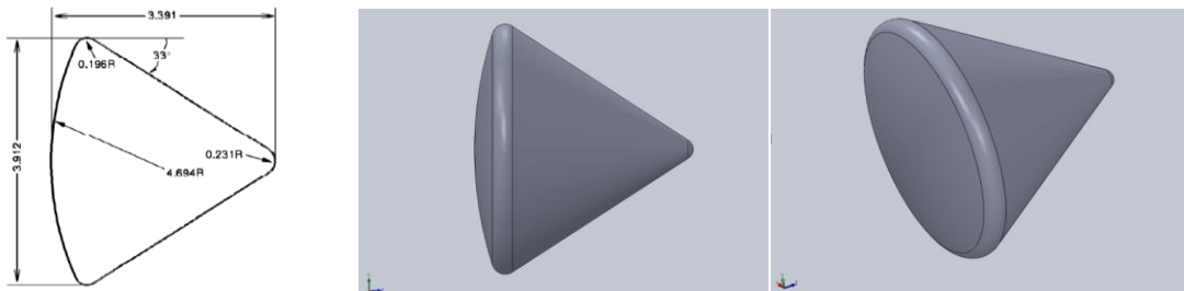
Figure 1: Dimension and solid model of Apollo AS-202 Command Module
